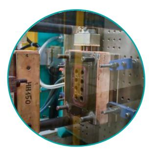
The production cycle of a silicone component is longer than that of a similar TPE component. The production equipment (moulds, machines, etc.) is more expensive. The investment can be offset by the production volume, as it is suitable for largescale production by injection moulding.
