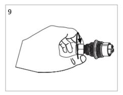
• Unscrew the pressure nut till it comes out from the connector housing (Fig. 9.1).
