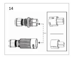
The male connector insert and the female connector insert can be inserted in both connector housings (male or female) depending on the application needs
