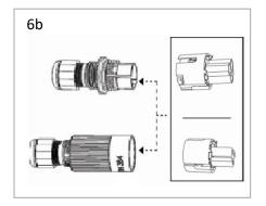
The female connector insert and the male connector insert can be inserted in both connector housings (male or female) depending on the application needs.
