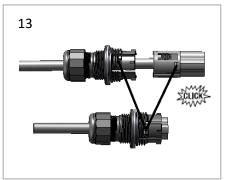
Insert the male connector insert in the housing until it stop. Make sure the connector insert's protrusion match with the housing's cavity
