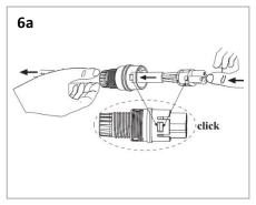
Insert the female connector insert in the housing until it stop. Make sure the connector insert's protrusion match with the housing's cavity
