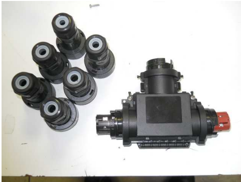
Connector model TH631 with 6 poles comply with § 15 and 16 of EN 60998-1:2004. (T=35°C, 24A, 2.5)
