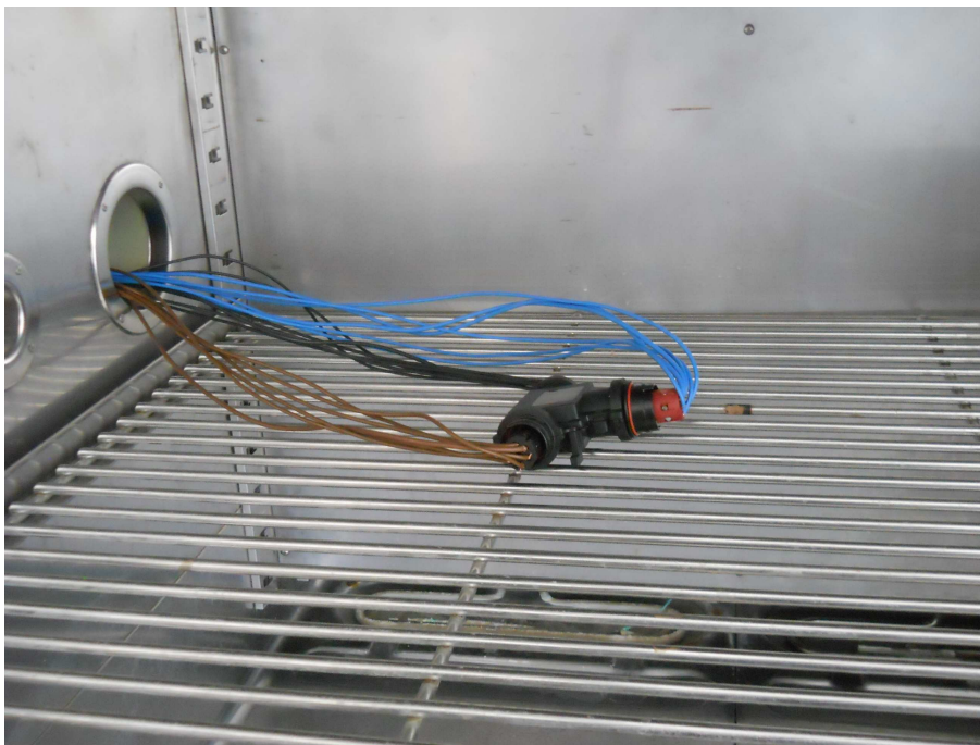
E.u.T inside climatic chamber
