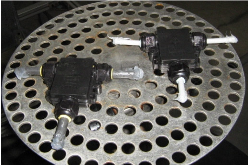
E.u.t. general view, same equipment with different section of cable Comply with IP67
