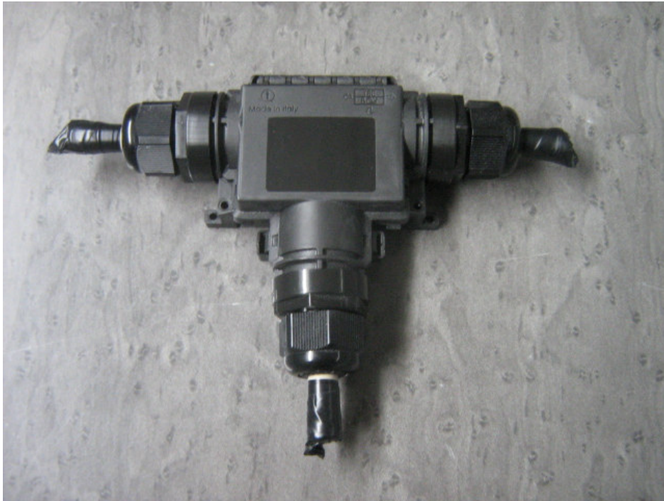
E.u.t. general view, same equipment with different section of cable Comply with IP65
