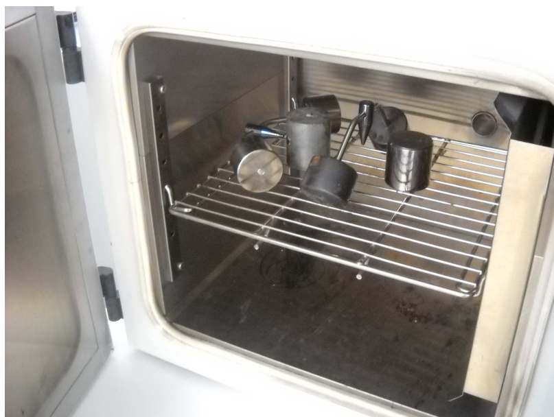
Foto No.6: Oven used for the Ball pressure-test
